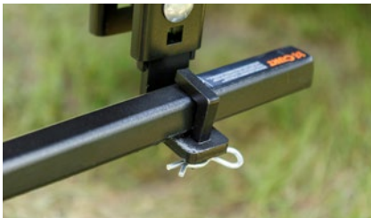
Two points of sway control use friction to distribute weight evenly, keeping trailer aligned
