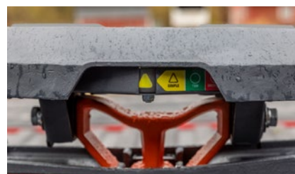
Three-position coupling indicator clearly shows coupling status
