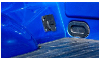
10' routes socket closer to truck cab
