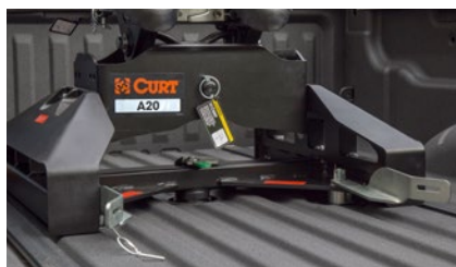
Step 1 - Drop OEM-compatible product into the truck bed puck system
