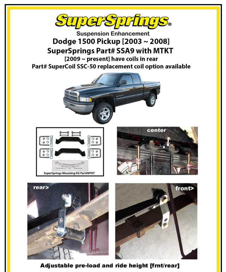
Refer to SuperSprings application guide for part selection www.supersprings.com [Tech line #866-898-0720] SuperSprings enhance load carrying capability, handling & towing. Never exceed vehicle manufacturer's GVWR rating.
