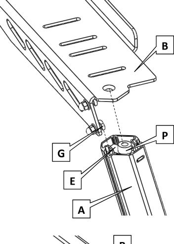
Align **(P)** 3/8-1.25" Flat Socket Bolt with the countersunk hole in **(B)** Left Bolt-On Brace ensuring **(P)** 7/16" x 1/2" Nylon Spacer stays in place on top of the Threaded Plate. Tighten Hardware.
