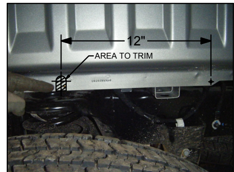
Figure 10.1: Inside Driver Side Rear Wheel Well
