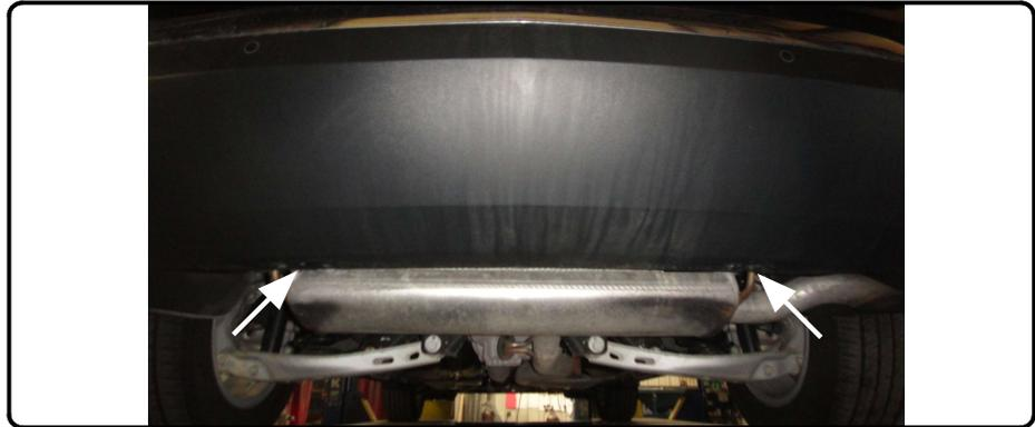
2. Lower the exhaust by removing the (4) bolts from each of the rear exhaust hanger brackets (2 per side) using a 15mm socket.
