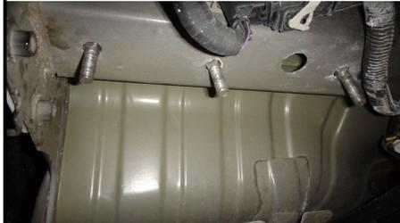
5. Raise hitch into position and secure the hitch to the vehicle using (6) 1/2" hex flange nuts.
