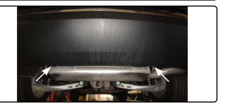
2. Lower the exhaust by removing the (4) bolts from each of the rear exhaust hanger brackets (2 per side) using a 15mm socket.
