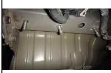
5. Raise hitch into position and secure the hitch to the vehicle using (6) 1/2" hex flange nuts.
