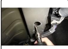
4. Utilizing the access hole, fishwire (1) 1/2" carriage bolt and (1) spacer into each of the three mounting holes in both frame rails.
