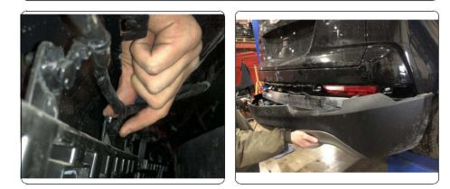
Remove bumper beam by locating and removing (4) fasteners on each side using 15mm socket. Unclip exhaust bracket from rear of vehicle to lower exhaust.
