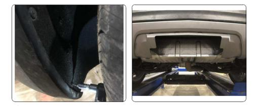
2. Pull back wheel well cover to remove (1) fastener using T-15 socket, on each side of vehicle. Carefully remove lower fascia, starting from outside and moving towards center on each side.
