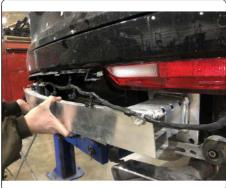
6. Reinstall exhaust bracket, using hardware removed in Step 4. Secure bracket, bumper beam, and hitch to
