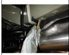
6. Reinstall heat shield and raise hitch into place and secure hitch to frame using the 1/2" hardware provided. Torque all hardware to 110 ft-lbs. Reinstall spare tire.
