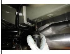
5. Fishwire 1/2" carriage bolt and spacer through the forward-most frame hole into the center and rear frame holes, then reverse fishwire into the forward-most hole for both sides.
