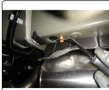
4. Trim heat shield to allow access to the front-center mounting holes. Enlarge the forward most mount hole to allow for 1/2" carriage bolt to fit through mounting hole.
