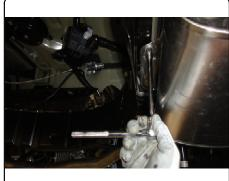
2. Locate and remove the center front attachment point on the spare tire shield using a 12mm socket. Remove the spare tire shield and return to the customer.
