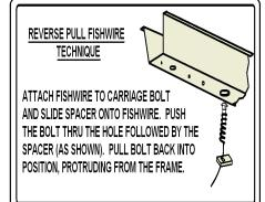
2. Fishwire (1) 1/2" carriage bolt and CM-SP6 spacer into the rearward most hole in both frame rails. Reverse fishwire the remaining hardware into the remaining holes in the bottom of the frame rails.
