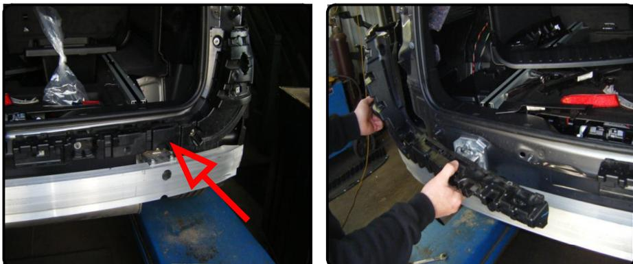
11. Remove bumper beam assembly by removing (4) nuts from threaded studs. These nuts will be used to install hitch.
