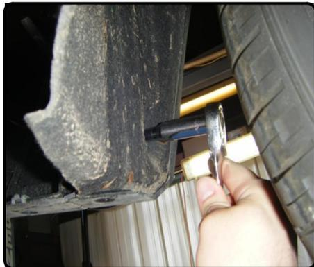
3. Remove (7) rivets from wheel well trim from above each rear tire. To remove rivets push small center rod through rivet with a small punch or an equivalent tool. Pry rivets from trim and pop trim off. **Note:** Replacement rivets are included.
