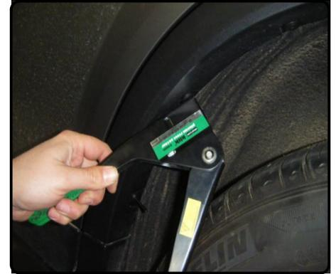
16. Raise underbody panel into position and mark the center using the hitch as a guide. Trim underbody panel. See UNDERBODY PANEL TRIM DIAGRAM on PAGE 2. Reinstall underbody panel and discard extra fastener. Install is complete.
