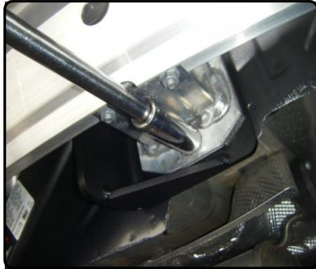
14. Hold inner plastic bodies in position and mark where the hitch side plates interfere. Trim an approximate 3/8" wide by 7/8" deep slot into each inner plastic body to allow for side plate clearance.
