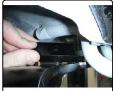
3. Slide the (2) 1/2" handle nuts into the grooved section of the frame over the forwardmost tabs and secure with 1/2" x 1 1/2" hex bolts and conical tooth washers. Slide the 1/2" x 5 1/2" hex bolts with washers through the frame and hitch brackets. Secure with 1/2" hex flange nuts.
