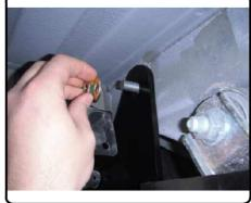
4. Torque all 9/16" fasteners to 150 lb-ft and all 1/2" fasteners to 110 lb-ft.
