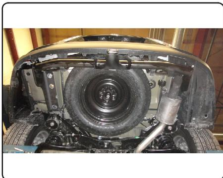
6. Mark and trim underbody panel. Reattach underbody panel using fasteners removed in Step (1). **Note:** See underbody panel trim diagram. Dimensions are approximate, confirm fit prior to trimming. Use ribs of the underbody panel as cutting guides.
