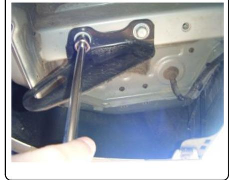
2. Lower rear most exhaust isolator for ease of installment.
