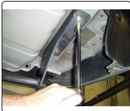
4. Raise exhaust back into location and reinstall rubber isolator.
