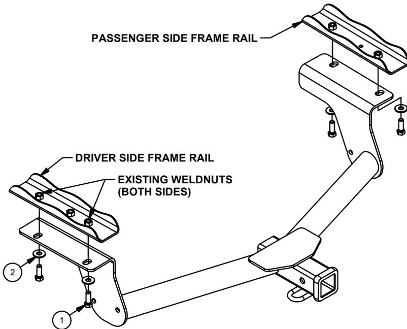
1. If present remove panel and trim using panel trim diagram below as reference. Remove the tie down bracket from the drivers side frame rail using the 17mm socket, 8" extension and ratchet. Return the bracket and fasteners to vehicle owner.
