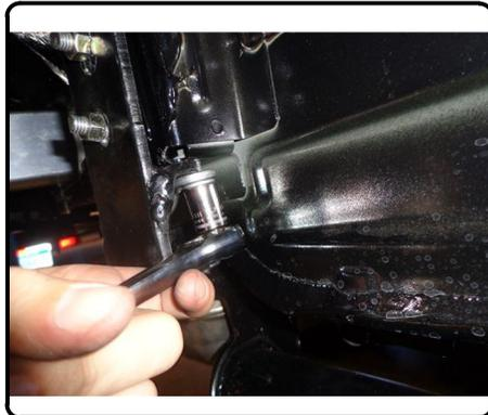
5. **Porsche models:** The trunk pan mounting holes must be drilled. Open trunk to clear vehicle components for drilling. Remove floor panels and spare tire, set aside. Disconnect battery terminals with a 10mm socket, remove audio module by removing (2) T-27 Torx screws. Disconnect battery strap using a 13mm socket and extension.
