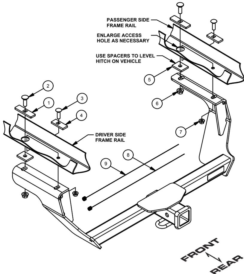
1) Remove the (4) plugs in the frame rails and discard (leave center plugs in).
