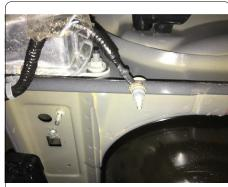
9. Raise hitch into position starting with the passenger side. Run the fishwires through the holes on hitch to help align bolts with hitch holes. Remove fishwires and loosely fasten (2) 1/2" hex nuts on driver side and (3) 1/2" hex nuts on passenger side.
