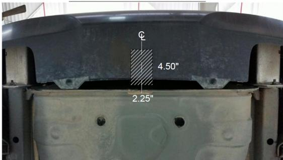
4. Raise hitch into position and loosely secure using existing vehicle hardware.
