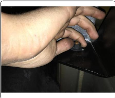
5. Use 15mm socket and torque all vehicle hardware to 45 ft-lbs. Reinstall pushpins removed in step 1.
